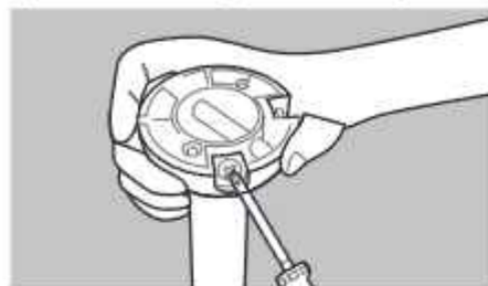
1 Loosen the screws on the hanging ball.
