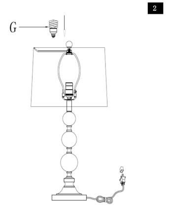
Step2 Insert the bulb(G) into the socket(C).
