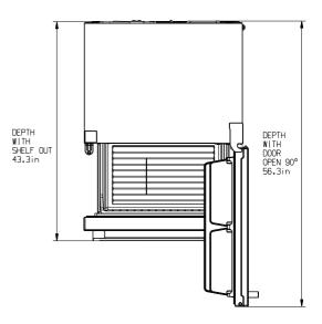
Keep enough clearance between the appliance and its surroundings to ensure the function of the appliance.
