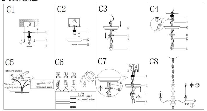
Step C1: .Attach the single bar (E) to outlet box with mounting screws (B). The side of single bar marked "GND" must face out Step C2: Raise the canopy (G) through screw collar loop (I) and screw the collar loop (I) to a proper position by measuring.
