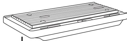
**2 A** Slide wrap onto base until it snaps into place.
