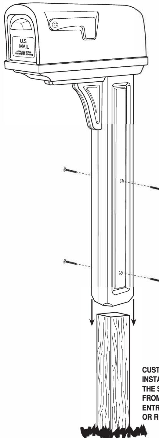
CUSTOMERS ARE REQUIRED TO CONTACT THE LOCAL POST OFFICE BEFORE INSTALLING THE MAILBOX TO ENSURE ITS CORRECT PLACEMENT AND HEIGHT AT THE STREET. GENERALLY, MAILBOXES ARE INSTALLED AT A HEIGHT OF 41-45 IN. FROM THE ROAD SURFACE TO INSIDE FLOOR OF THE MAILBOX OR POINT OF MAIL ENTRY (LOCKED DESIGNS) AND ARE SET BACK 6-8 IN. FROM FRONT FACE OF CURB OR ROAD EDGE TO THE MAILBOX DOOR.
