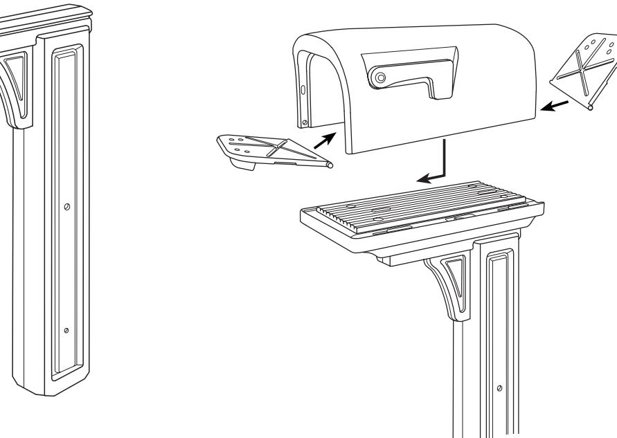
**3** **Dig a hole and install 40"- 48" treated 4x4 post (not included.)**
