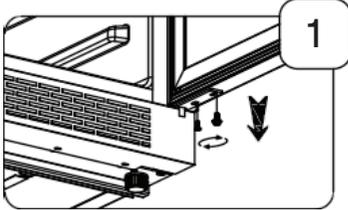
1. Open the door and using a Phillips screwdriver, remove the bottom screws from the lower hinge.
