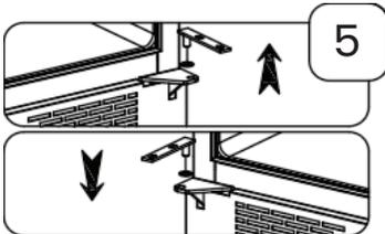
5. Remove the door axis from the lower right hinge. Install the door axis on the lower left hinge.
