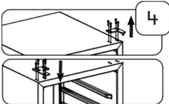
4. Remove the screws from the upper right hinge. Place the upper right hinge in a safe place in case you need to reverse the door in the future. Remove the decorative covers from the upper left hinge corner. Install the upper left hinge by fastening the screws through the left hinge to the cabinet. Insert the decorative covers to the upper right hinge. Insert the silver plastic cover to the bottom hinge of the door.
