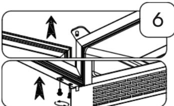
6. Carefully insert the door into the upper left hinge, then slide the door on top of the lower hinge and secure the door by installing the lower screws.
