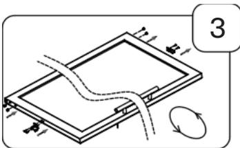
3. The door revolves 180 degrees. Remove the door magnet and install it on the opposite side. Remove the silver plastic cover from the top hinge of the door.
