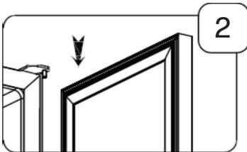
2. Pull down to remove the glass door and place it on a padded surface to prevent scratching it.
