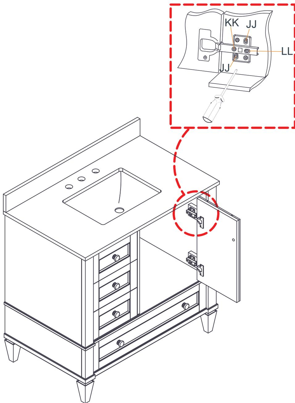
Uneven floor may cause doors to hang incorrectly. Please place the vanity on level surface, or adjust the levelers at the bottom to ensure that it is perfectly level. If necessary, doors can be adjusted with a Philips screwdriver at the adjustable hinges.
