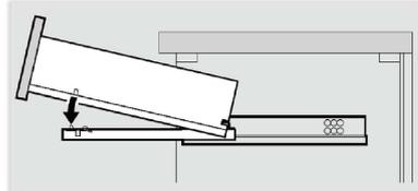
Pull forward until the peg engages with the fixing holes in the drawer base.
