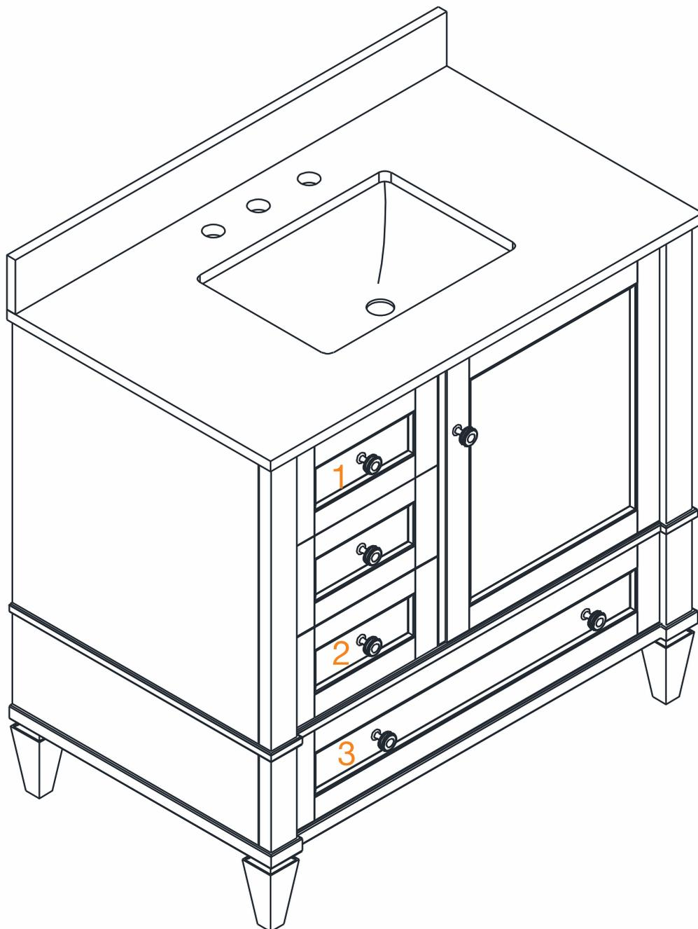
In case drawers need to be removed, each drawer is individually numbered underneath the drawer box with the corresponding number on top of the dust partition, inside the case.
