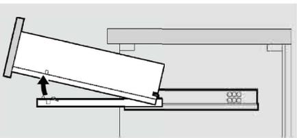
Pull the peg out of the fixing holes in the drawer base.
