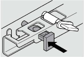
Lock the peg by pushing inside the hole in the drawer base side.
