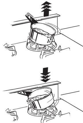
**IMPORTANT:** If the vent is obstructed by an object while it is being raised or lowered, it will stop. Remove the obstruction and press the **ON/OFF** pad again.
