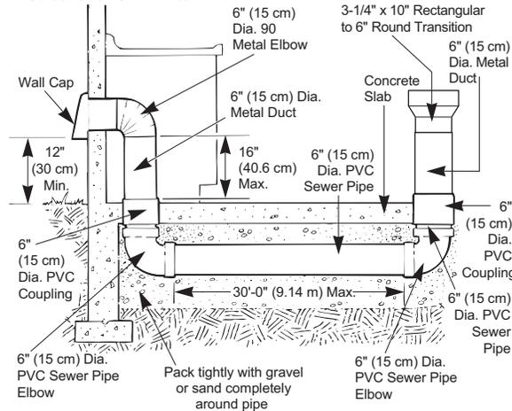
Install ductwork so the piece of duct nearest the downdraft unit slots INTO the next piece of the duct. Secure the joints with self-tapping screws and apply duct tape around the joints to ensure an airtight seal.
