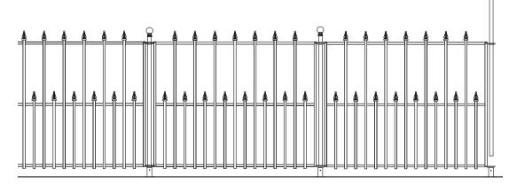
Continue adding panels, using the panel to mark the position of the next stake
