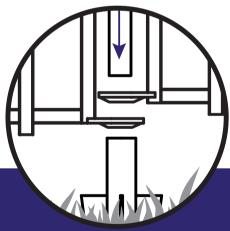
Hint: Drop post through panel rings to mark the placement for the next stake
