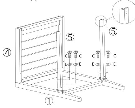
3 Connect the rear leg 2 and tighten to 80%.
