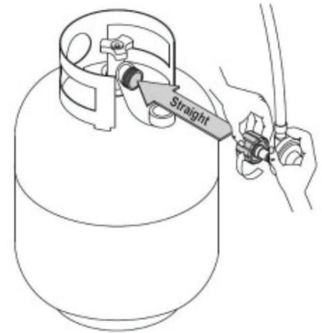
**! WARNING:** The Type I connective coupling (see Fig. 4) supplied with your grill must not be replaced with a different type of grill/tank connection system. Removal will result in loss of warranty, gas leakage, fire and severe bodily harm.
