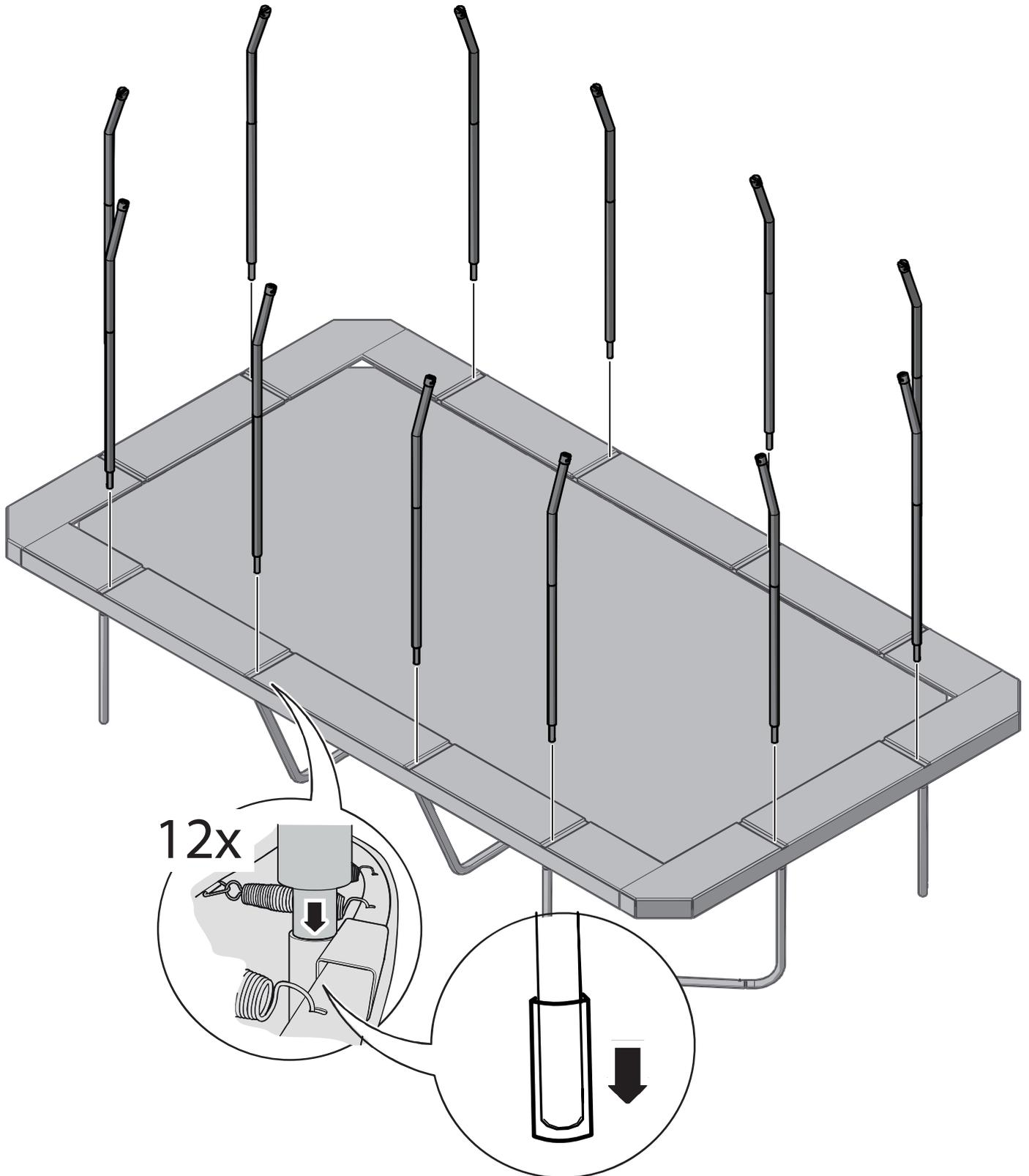
Please make sure the pole completely inserted into T-connector+welded tube.
