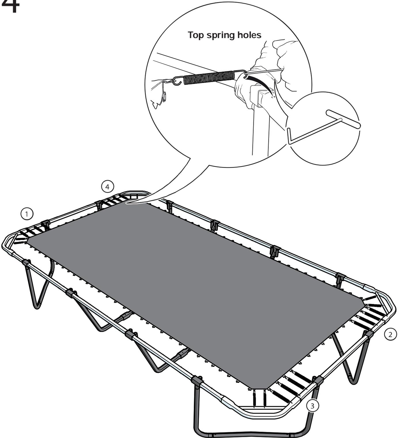
Next you will use 16 8.5" springs and place 4 into top spring holes in the frame in position 1, then 2 (diagonally across), then 3 & finally 4 (diagonally across).
