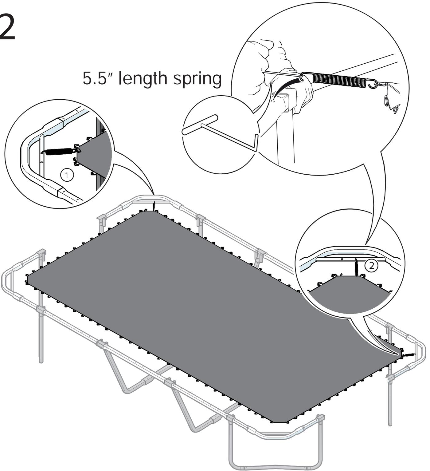
Then take 4 of the 5.5" springs and use the spring pulling tool to insert one end into trampoline frame after connecting the other end to the V-ring. Place in the 1st corner than go to the next corner and repeat this step.
