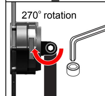
1. Use the Allen key to tighten and loosen the connection between the arm and the holder, adjusting ease of rotation in the tablet holder.
