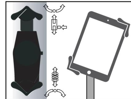
Press button on side of tablet holder to slide open. Insert your tablet against spring arm. Slide other end back to secure device.
