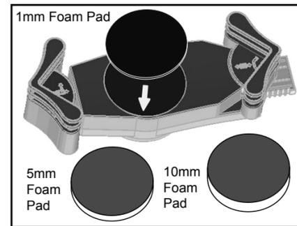
Select the appropriate foam pad according to the thickness of your tablet or case. Press adhesive side into center of tablet holder.
