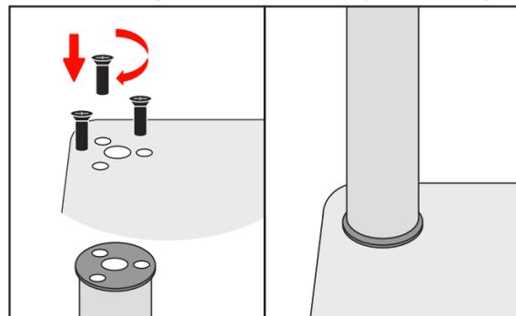
1. Align the pole and plate using the three holes. Screw them together from the bottom up using included screws.
