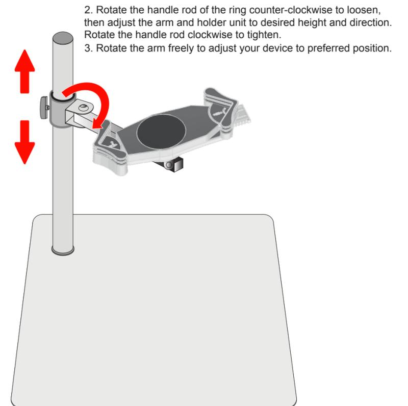
2. Rotate the handle rod of the ring counter-clockwise to loosen, then adjust the arm and holder unit to desired height and direction. Rotate the handle rod clockwise to tighten.
