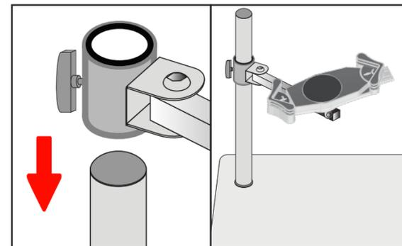
2. Go through the ring of the Arm and Holder unit to the pole. Place it at your preferred height then turn the handle rod to tighten.
