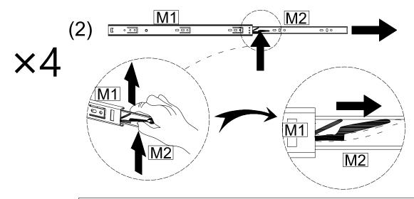
Move the black paddle upward and pull out (M2) to the right.
