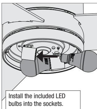
Install the included LED bulbs into the sockets. When necessary, replace with bulbs of same wattage.
