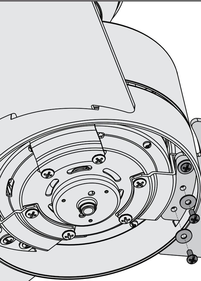
Attach each blade to a blade iron using three blade washers, found in the ■ hardware bag, and three blade assembly screws, found in the ▲ hardware bag.
