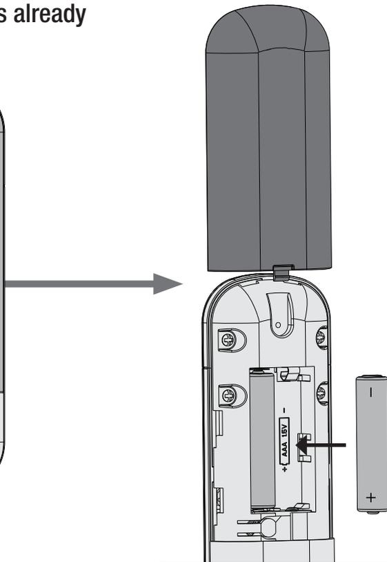
Install two AAA batteries, found in the remote control hardware bag, into the transmitter. Clean the battery contacts prior to installing the batteries. Please contact your local battery recycling center for proper battery disposal information.
