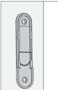
Press the cradle bracket against the wall and hold firmly for 30 seconds.
