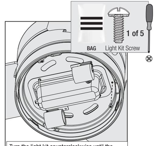
Turn the light kit counterclockwise until the switch housing screws are firmly situated in the narrow end of the keyhole slots. Install the third screw and tighten all three screws securely.
