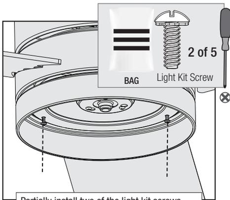
Partially install two of the light kit screws found in the hardware bag. It does not matter which two screw holes you choose.
