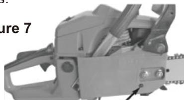
3) Turn the screw to the right to increase the tension and turn it to the left to release tension.
