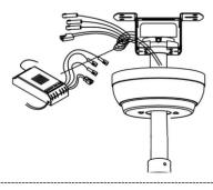
☐ Insert the receiver into the mounting bracket with the flat side of the receiver facing the ceiling
