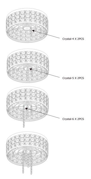
Repeat the above step 8 times to complete the outer ring crystal hang
