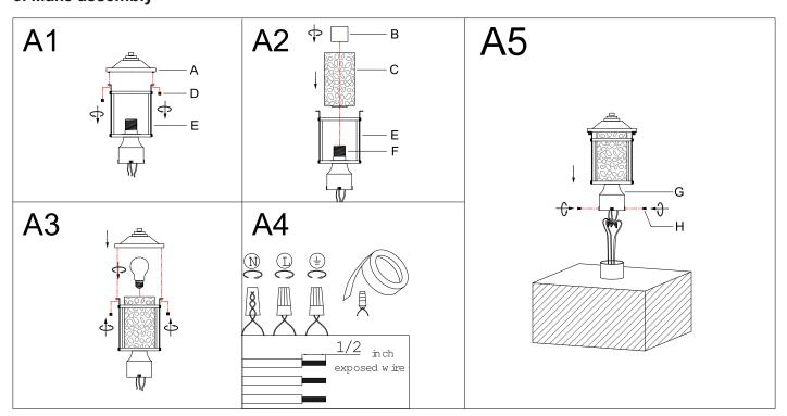
Step A1 » Unscrew knob nuts (D) from lid (A) and frame (E), then set them aside for later installation.
