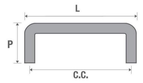
C.C = Center to Center (Distance between the drill holes)
