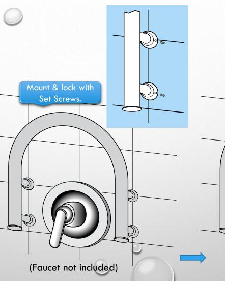
To check secure mounting, pull the U-Shape Bar slightly.
