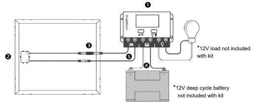
Remove the panel covering. In good sunlight, the charge controller's • "BAT %" should increase to 100%. Once the battery is fully charged and the controller is set to "LOAD ON," the system will provide power through the load control output or through the two USB ports. If an inverter is added to the system, it must be connected to the battery bank, and not to the charge controller.
