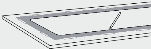
2. Cut the countertop using the appropriate cutting tools. Cutting on the line will result in a flush installation. Adjust the line accordingly if a positive or negative reveal is desired. If using a CNC machine, download the DXF file from [www.lowes.com](http://www.lowes.com) and proceed accordingly.
