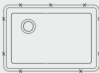
3. Turn the sink upside down. Align the sink with the cutting line on the counter. Using a pencil, mark 10 spots around the rim at a distance of about 3/4 in. to 1 in. from the edge of the sink. For a solid installation, it is recommended that all included mounting clips are used.
