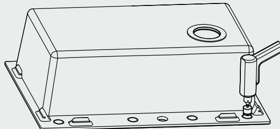
5. Attach the supplied clips to the anchor points on the underside of the sink rim. Lightly hammer if needed.
