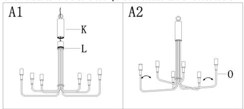
Step A1: Slip tube (K) over the wires and then thread it into the top of fixture loop (L).
