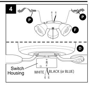
5. Connect WHITE wire from switch housing to WHITE wire from light kit fitter (F). Connect BLACK (or BLUE) wire from switch housing to BLACK wire from light kit fitter (F). Make sure molex connections are secure.
