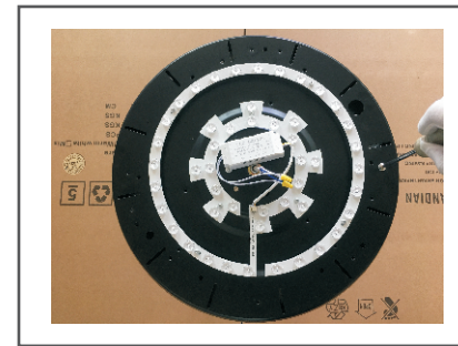
Step 4. Remove the main engine chassis screws.
