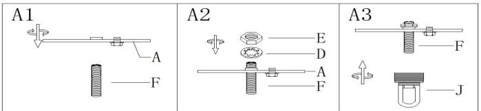
Step A1: Thread the single bar(A) onto the nipple (F), At this point need note that: the side of single bar marked "GND" must
