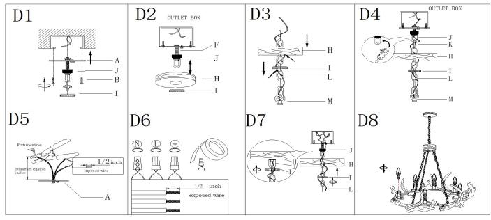
Step C1: Remove the threaded ring (I) from collar loop(J).
