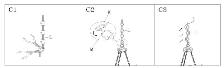
Step C1: By measuring, determine the correct number of links needed for proper hanging height. Using the chain pliers, disconnect and discard the remaining chain.
