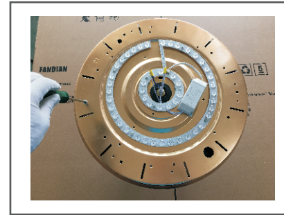
Step 4. Remove the main engine chassis screws.
