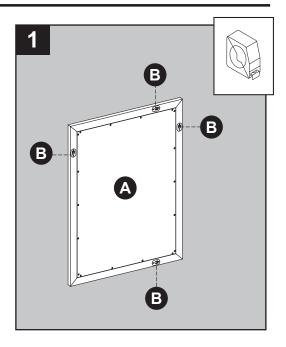
2. Measure and mark location for mounting hardware on the wall using the measurement from Step 1. Make sure the marks are level and located at the desired height.
