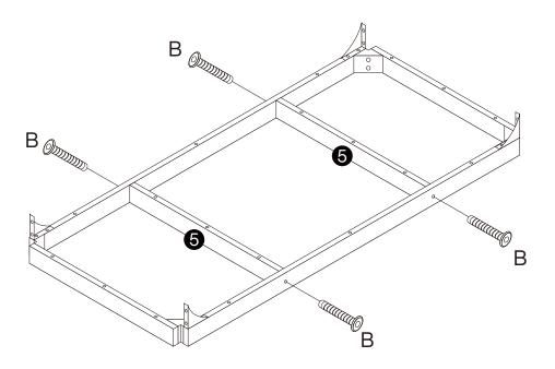
Friendly Tips: Do not fully tighten all screws until assembly is completed.
