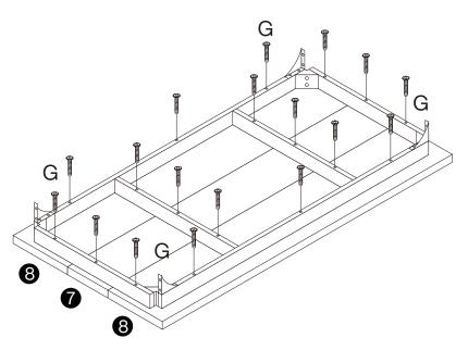
Friendly Tips: The screws used to connect the desktop to the steel frame only need to be tightened to the bottom of the screws and rotated once!
