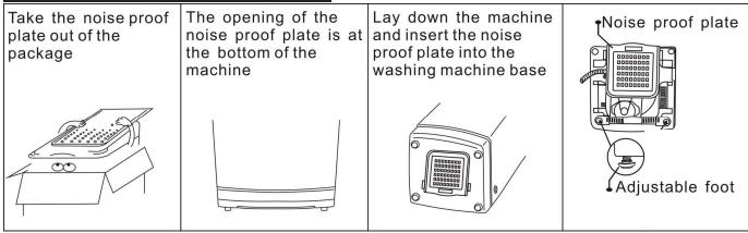
Affix the noise proof plate by using the two screws provided.
