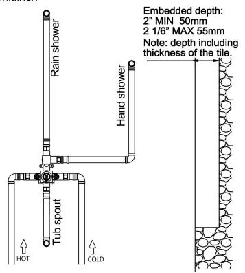
5. Install the upper outlet pipe and the top shower head. (wrap the PTFE tape on the thread)
