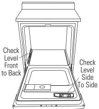
• Level the dishwasher by adjusting the four leveling legs individually.
