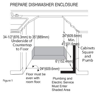
· The rough cabinet opening must be at least 24"(609.6mm) deep and to 24"(609.6mm) wide. The opening should be to 35" (889mm) max height.
