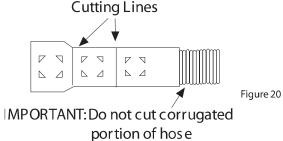
• If a longer drain hose is required, add up to 42" (1067mm) length for a total of 10ft.(3.05mm) to the factory installed hose. Use 5/8"(15.9mm) or 7/8"(22M) inside diameter hose and a coupler to connect two hose ends.. Secure the connection with hose clamps.
