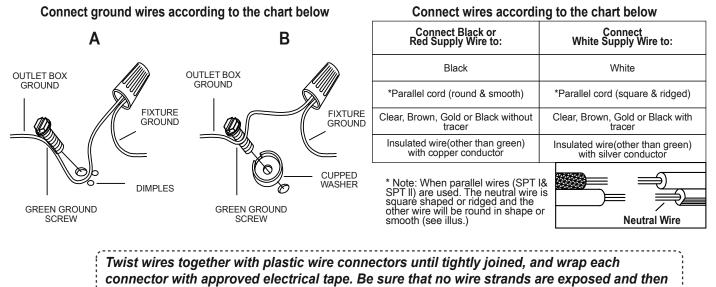
carefully tuck all wires into the outlet box.
