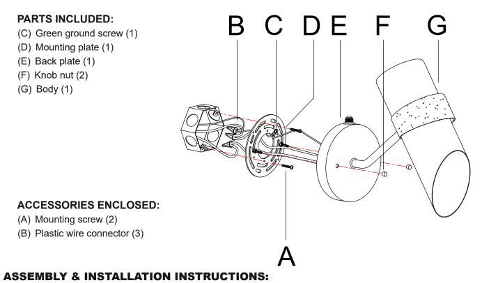
1. Carefully remove the fixture from the carton and check that all parts and accessories are included as shown in the above illustration.
