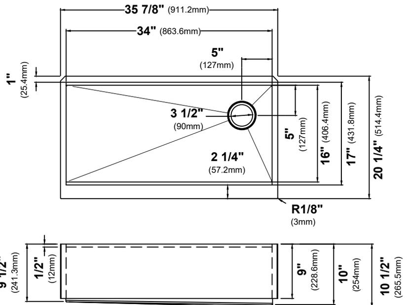
**NOTE:** It is not recommended to install this sink with a negative reveal. Doing so will prohibit the use of any workstation accessories as they will not fit.
