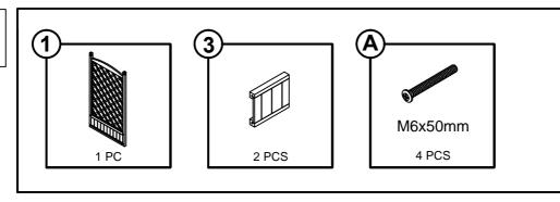
STEP 1: Locate Trellis (1) and attach Side Panels (3) with four blot (A).
