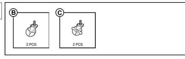
STEP 3: Attach the Casters (B) to the front of the planter base. Repeat with the Locking Casters (C) and attach them to the planter base.
