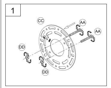
1. Loosely thread the screws (AA) and the hex nuts (DD) onto the round mounting plate (CC).
