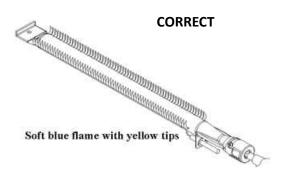
■ To adjust air shutter, loosen set screw and rotate air shutter to desired position to achieve normal flame. Tighten set screw after adjustment is made. Relight the pizza oven to observe flame. Incremental adjustments may be needed to achieve a good Flame.
