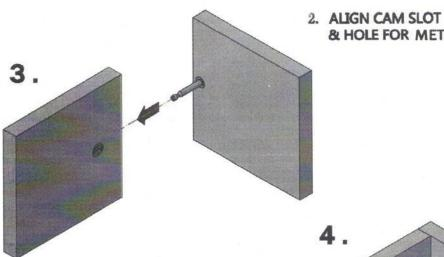
3. Install Metal Dowel (ee) into Cam outer ring before installing center of Cam into Cam outer ring(to prevent center of Cam blocking Dowel)
