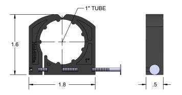
HOLDRITE #181, #182 & #183 Full S-Nail Clamps are ideal for "Surface Mounted" positioning of 1/2", 3/4" & 1" CTS tubing (Copper, CPVC or PEX). The nail is preloaded into the clamp for quick installation. Provides protection against tubing damage caused by abrasion or contact between dissimilar metals.
