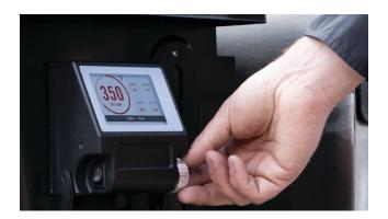
9. When the startup cycle is finished the controller will display the temperature and the lid can be closed, allowing the pellet grill to reach and maintain the set temperature.
