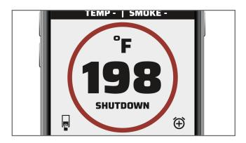
16. Select SHUTDOWN from the main menu. In this setting the fan will remain on for 20 minutes to finish burning any pellets in the burn cup.
