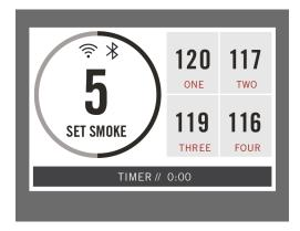
A smoke setting of 1 will produce less smoke and maintain a more even temperature. As the smoke setting increases, the temperature fluctuations will also increase.
