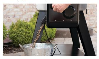
Empty the pellet hopper to prevent your pellets from getting wet or coming into contact with cleaning substances.
