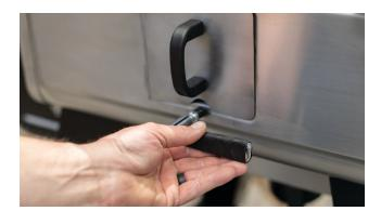
3. Rotate the valve handle to the horizontal position to allow flames into the smoke box. Once the wood/charcoal has started, rotate the valve handle back to the vertical position to smoke.
