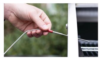
12. Insert the probe and wire through the stainless flap on the side of the chamber.
