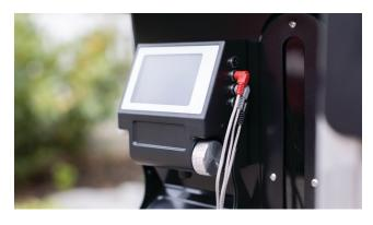
11. Plug the probe into one of the four available ports on the controller.
