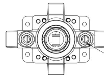
It can close water when you screw clockwise slotted screwdriver on both sides
