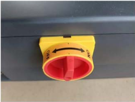
A. The power switch rotates clockwise. ON-Turn on OFF-Turn off
