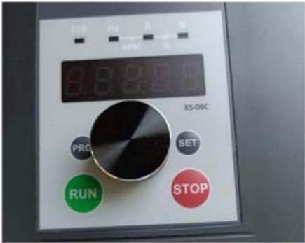
B. Controller panel operating instructions RUN-Run button STOP stop button
