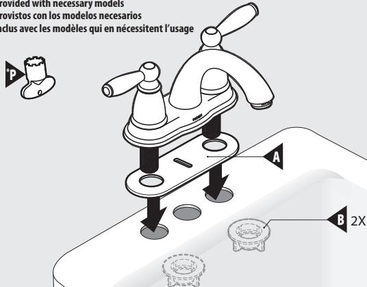
Note: Spout, handles, gasket and lift rod vary by model.
