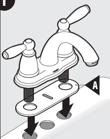
After removal of old faucet, clean and dry the sink surface. Install faucet with gasket (A). Some gaskets are preinstalled and shape will vary by product.
