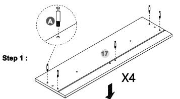
The long groove is used to install the bottom plate, make sure to take note of installing the grooves of these boards on the same side.
