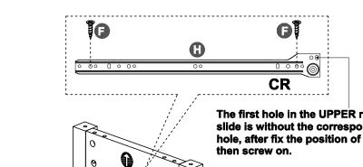
The first hole in the UPPER row holes of the slide is without the corresponding pre-drilled hole, after fix the position of the slide and
