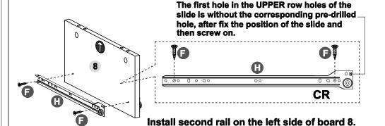
NOTICE:To ensure the stability of the structure, please pay attention to the hole position when locking screws.CL slide should lock on the first hole position near the pulley, CR slide lock on the second hole position near the pulley.
