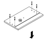
The long groove is used to install the bottom plate, make sure to take note of installing the grooves of these boards on the same side.
