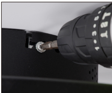
4. Loosen the four remaining screws from the "L-shaped" holes on each side of the canopy.
