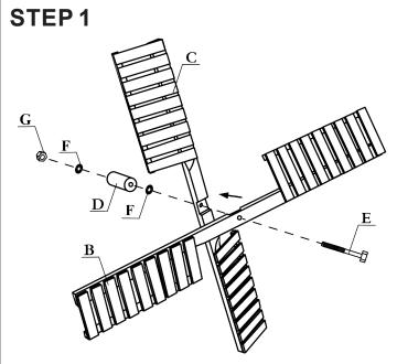
Place Front Blade (B) onto Back Blade (C) as shown. Slide Bolt (E) through the blades, Washer (F), Shaft (D), Washer (F), and Nut (G). Hand-tighten the bolt. **Do not over-tighten the hardware.**
