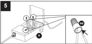
Using wire nuts(BB),connect supply cable to hardwire junction box(B) in the following manner: green to ground, white to white, black to black. Place all wiring connections back into the hardwire junction box (B) and close the cover.
