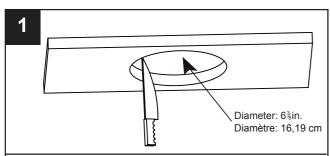
Locate a suitable location for the fixture and cut a 6% in round hole where the LED Ultra-Thin Downlight(A) will be installed. Ensure this location has access to electrical wire from the switch (power supply).
