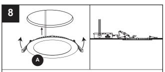
Push the spring loaded clips on the LED Ultra-Thin Downlight(A) upwards and insert the base of the LED Ultra-Thin Downlight(A) into the mounting hole established in Step 1.Release the clips and the fixture will grip flush with the ceiling/drywall.
