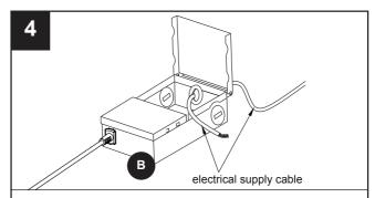
Insert the electrical supply cable through the knockout and secure with a cable connector(sold separately).
