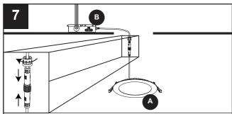
Connect the LED Ultra-Thin Downlight (A) to the hardwire junction box(B) by inserting and twisting the male/female connections of the attached connector cables together.
