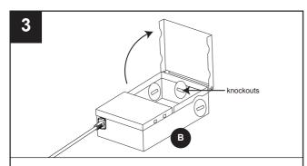
Carefully open the hardwire junction box (B)and remove the appropriate knockout(s).
