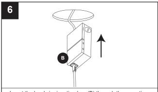
Insert the hardwire junction box (B) through the mounting hole established in Step 1.
