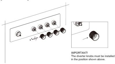
7. Insert the push button connectors into the knobs and secure.
