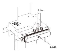
2. Wrap telon tape around the threads of the male adapters and connect the hot, cold, shower head, and hand shower water lines to the valve body.
