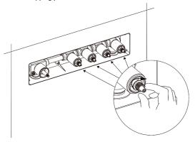
5. On the back side of the valve trim panel, run a bead of silicone around the edge and place it onto the valve body securing it to the finish wall.
