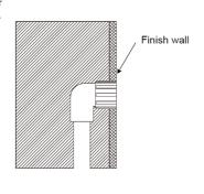
13. Wrap the threads of the hand shower arm connector and screw it into the wall connection, as shown in the images.
