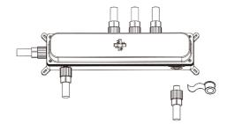
3. After the wall is finished, remove the plastergaurd from the valve body and cut the valve body casing flush with the wall if necessary. Discard the platergaurd.
