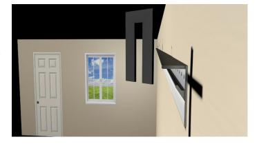
c. Adjusting for high spots in the wall. This is not done now but rather is accomplished when mounting the cabinet brackets. You simply note where on the wall that the high spot is located in the cabinet arrangement, identify the affected cabinet, and then adjust the location of the
