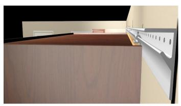
d. The location of the corner cabinet brackets at A will allow for the alignment of the adjacent cabinets on the walls in either direction. Once the corner cabinet is in place you can check the clearance between the cabinet and rail throughout the corner. If the walls are square, you can add other brackets at location B as in the diagram below. If the walls are out of square, you may only be able to attach
