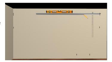
e. Let the wall rail pivot downward to a resting point while locating the centers of the rest of the wall studs along the line just drawn.
