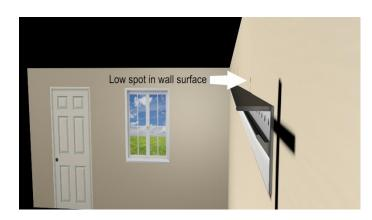
b. Loosen the rail attachment screws in these low areas and insert the provided plastic horseshoe style shims between the rail and the wall at the stud locations as needed to align the top of the rail in a straight manner. After shims have been added, all of the rail mounting screws should be tightened securely. Re-check the wall rail for straightness and levelness.
