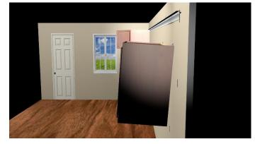
b. The cabinet will move slightly away from the wall and then will quickly move toward the wall at which point you can stop the upward motion, allowing the brackets to engage the wall rail.
