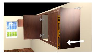
b. Drill 3/16" holes through the cabinet just above the bottom interior surface of the cabinet in alignment with the wall studs.
