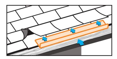
Fasten with 3 hot dipped galvanized roofing nails.
